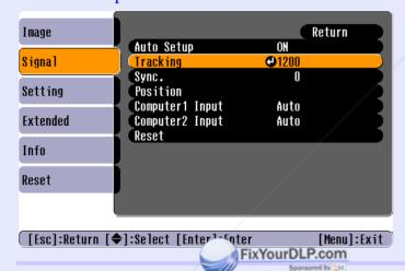
Tilt the [♠] button on the remote control or press the [♠] and [▷] buttons on the projector's control panel to adjust the tracking value until the vertical stripes disappear from the images.
