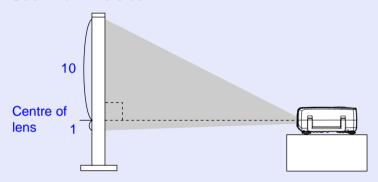
If it is not possible to set up the projector so that it is perpendicular to the screen, it can be set up at a slight vertical angle instead. You can adjust the upward projection angle of the projector to a maximum of 12° and the downward projection angle to a maximum of 4° by extending and retracting the front adjustable foot and rear adjustable feet.
