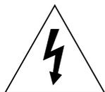
The lightning flash with arrowhead symbol, within an equilateral triangle, is intended to alert the user to the presence of uninsulated “dangerous voltage” within the product’s enclosure that may be of sufficient magnitude to constitute a risk of electric shock.
