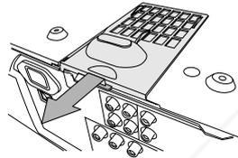
2. Remove the air-filter from the filter cover.
