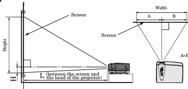
To find the approximate distance between the projector and screen: Multiply the width of the screen x 1.8 (min.), Multiply the width of the screen x 2.3 (max.).
