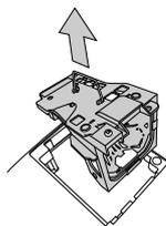
5. Hold onto the projector by the handle as you pull out the lamp.
