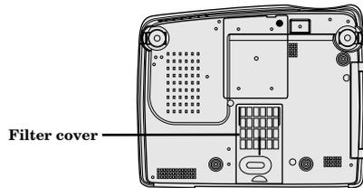
1. To remove the filter cover, slide the cover in the direction of the arrow.
