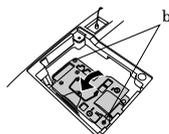
9. Tighten up the screws of the lamp lid using a Phillips screwdriver (+).
