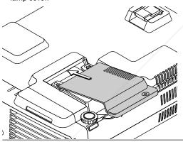
(2) Turn the lamp cover's screw clockwise to tighten it.
