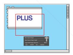
(2) Press the "+"/"-" buttons and determine the capture size. The lower right (end point) will move. To switch between height and width, press the MENU button.
