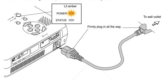
2 Switch on the projector power Projector operation: Press the POWER button.
