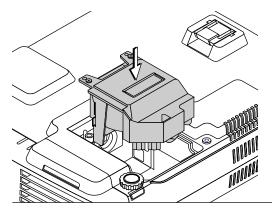
(2) Turn the two lamp cartridge screws clockwise to tighten them.
