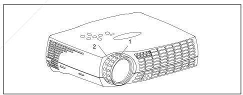
Turn the focus ring (1) to adjust the picture sharpness. FixYourDifference to the zoom ring (2) to adjust the picture size. DISCOURT TO THE TRUSTED SOURCE FOR PROJECTOR LAMPS AND ACCESSORIES THE TRUSTED SOURCE FOR PROJECTOR LAMPS AND ACCESSORIES
