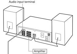
ø3.5 mm stereo minijack to RCA audio cable (commercially available)
