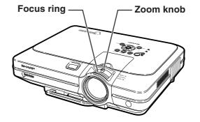
**1** The focus is adjusted by rotating the focus ring.
