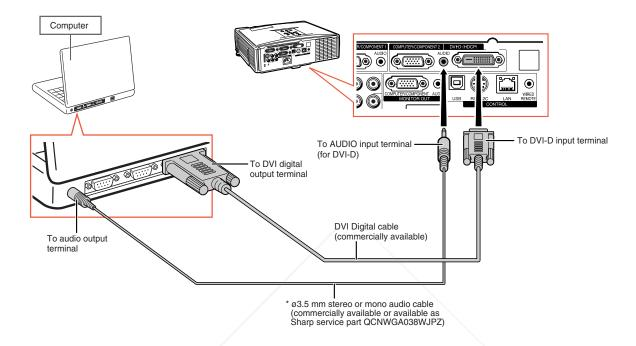
\* When using the ø3.5 mm mono audio cable, the volume level will be half of when using the ø3.5 mm stereo audio cable.
