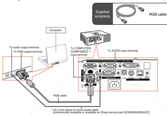
\* When using the ø3.5 mm mono audio cable, the volume level will be half of when using the ø3.5 mm stereo audio cable.
