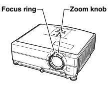
1 The focus is adjusted by rotating the focus ring.
