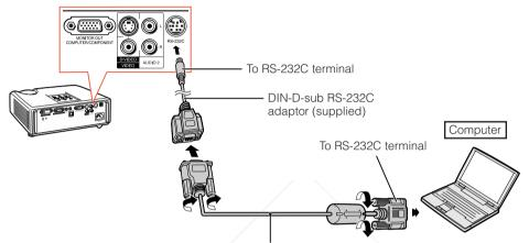
RS-232C serial control cable (cross type, commercially available)
