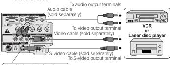
Use this terminal when the audio-visual equipment to be connected has an S-VIDEO output terminal.
