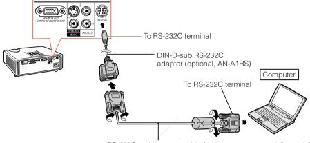
RS-232C serial control cable (cross type, commercially available)
