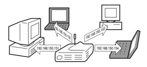
Make the following settings when using this function Set the DHCP server function on the projector to ON
