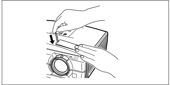
**2 Slide the lens fastener catch tab in the direction of “UNLOCK” while holding the lens to prevent it from falling out.**
