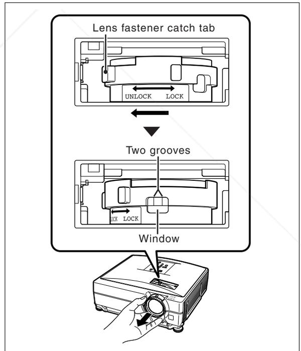
**3 Remove the lens by pulling it straight out.**
