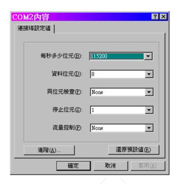
After settling down, connect our specific RS232 cable and press the 'call' icon of 'Hyper Terminal' program. After this, press 'Enter' key, if an '>' symbol come up, that means the unit is ready to accept commands for computer.
