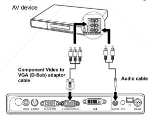
The projector is only capable of playing mixed mono audio, even if a stereo audio input is connected. See "Connecting audio" on page 16 for details.
