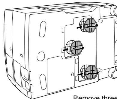
Remove three Air Filters by pulling up the latches.
