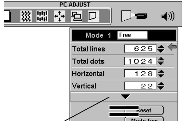
Press the SELECT button at this column to adjust "Clamp," "Fine sync," "Display area," "Horiz. scale" or "Vert. scale" .
