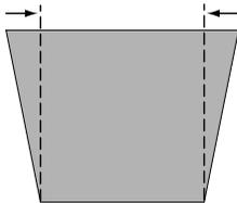
Reduce the lower width with the KEY STONE ▼ button or the POINT DOWN button.
