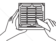
The air filter is set in the reverse side
