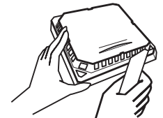
The air filter is set in the reverse side
