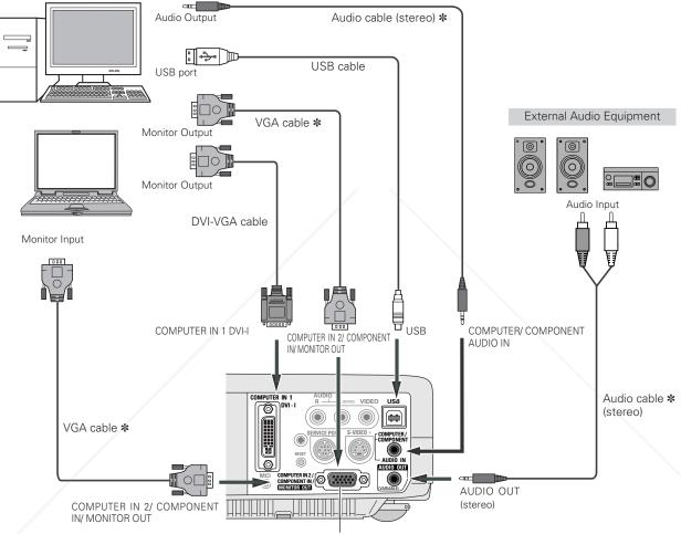
This terminal is switcheable. Set up the terminal as either Computer input or Monitor output. (See Page 44.)
