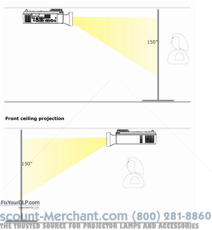
A special method of installation is required in order to suspend the projector from the ceiling. Please ask your dealer for details.
