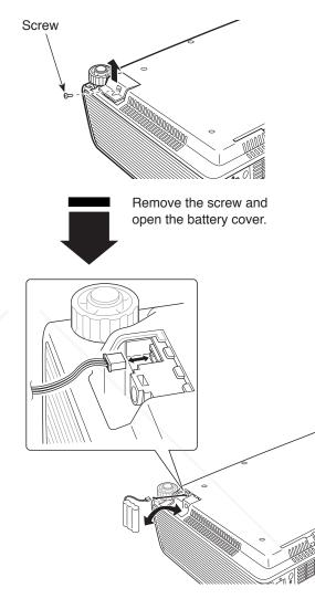
Install the battery, then put back the battery cover and secure it with the screw.
