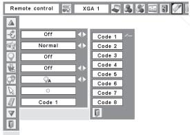
While holding down the MENU button, press the IMAGE button the number of times corresponding to the remote (800) 281-8860 control code for the projector. See "Remote Control Code" on page 15. SOURCE FOR PROJECTOR LAMPS AND ACCESSORIES
