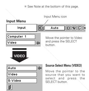
When video input signal is connected to the VIDEO Video Djack, select Video.
