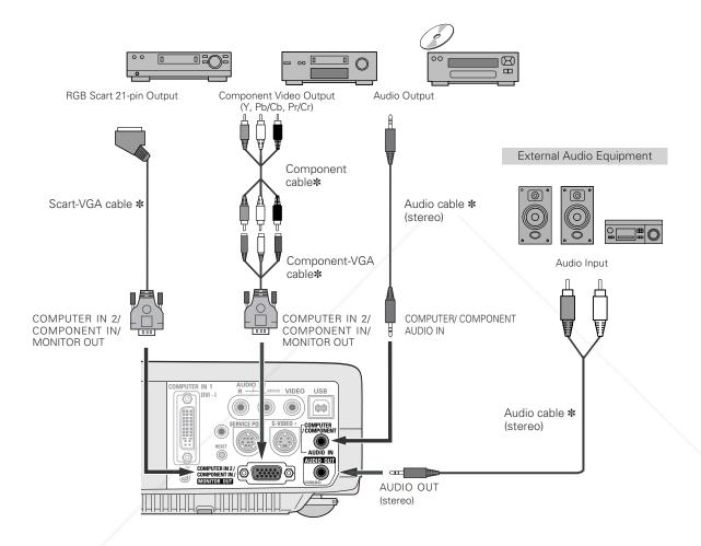
• Input sound to the COMPUTER/COMPONENT AUDIO IN terminal when using the
