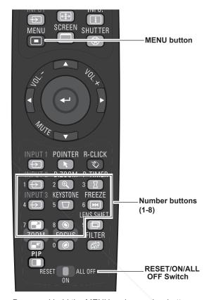
Press and hold the MENU and a number button (1-8) that corresponds to the remote control code for more than five seconds to switch between the codes.
