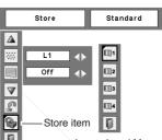
Image Level Menu Move the red framed pointer to an image item to be set and then press the SELECT button
