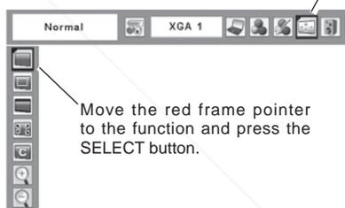
Move the red frame pointer to the function and press the SELECT button.
