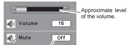
Press the MUTE button to set the Mute function On/Off. The display disappears after 4 seconds.
