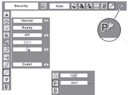
When the projector is locked with the PIN code, the PIN code lock mark appears on the menu bar.
