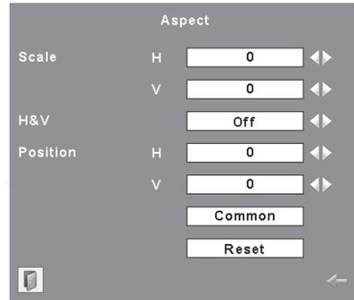
Scale H/V ..... Adjust the Horizontal/Vertical screen scale.
