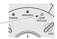
This indicator lights yellow when the life of the projection lamp draws to an end.
