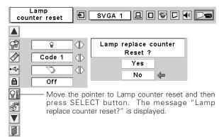
Note: Do not reset the Lamp Replace Counter until after the projection lamp is replaced.
