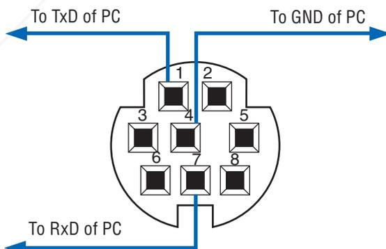
*NOTE: Pins 2, 3, 5, 6 and 8 are used inside the projector.*
