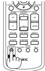
If the projector can be operated with the current remote control ID, the [ACTIVE] will be displayed. If the projector cannot be operated with the current remote control ID, the [INACTIVE] will be displayed. To operate the inactive projector, assign the control ID used for the projector by using the following procedure (Step 3).
