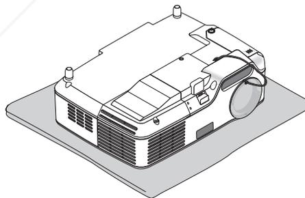
2. Loosen the lamp cover screw until the screwdriver goes into a freewheeling condition and remove the lamp cover.
