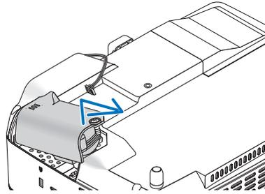
**NOTE:** Keep the contact area of the connector clean. If there are dust and dirt in the contact area of the connector, remove them.
