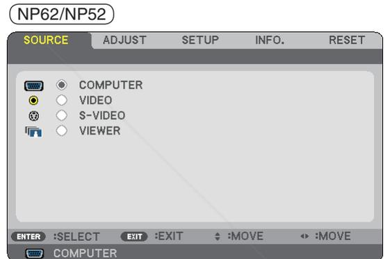
2. Press the SELECT ► button to select [SETUP] and press the ENTER button.
