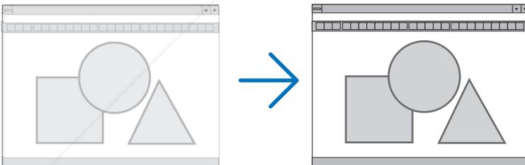
**PHASE**..... Use this item to adjust the clock phase or to reduce video noise, dot interference or cross talk. (This is evident when part of your image appears to be shimmering.) Use [PHASE] only after the [CLOCK] is complete.
