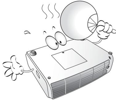
2. Do not operate lamps beyond the rated lamp life. Excessive operation of lamps beyond the rated life could cause them to explode on rare occasions.
