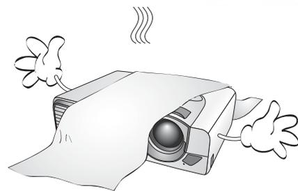
If the ventilation holes are seriously obstructed, overheating inside the unit may cause damage to the lamp, the projector to fail or result in fire.
