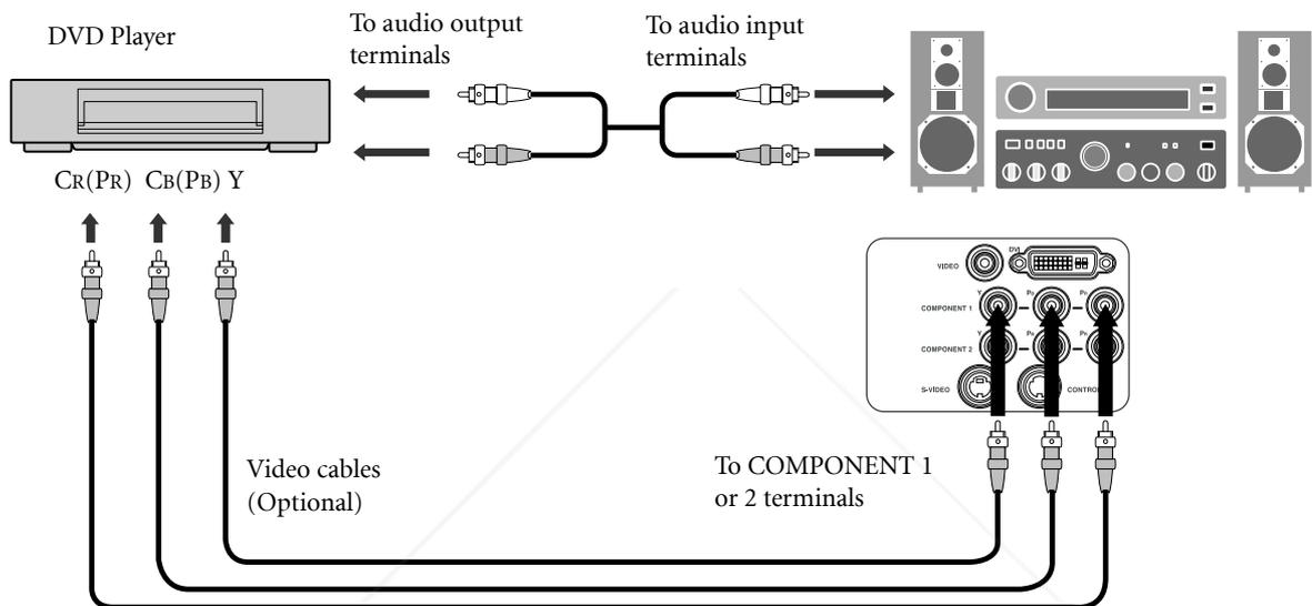
**ⓘ** If the selected video images is not displayed after the projector is turned on and the correct video source has been selected, please check that the video source is turned on and operating correctly. Also check that the signal cables have been connected correctly.
