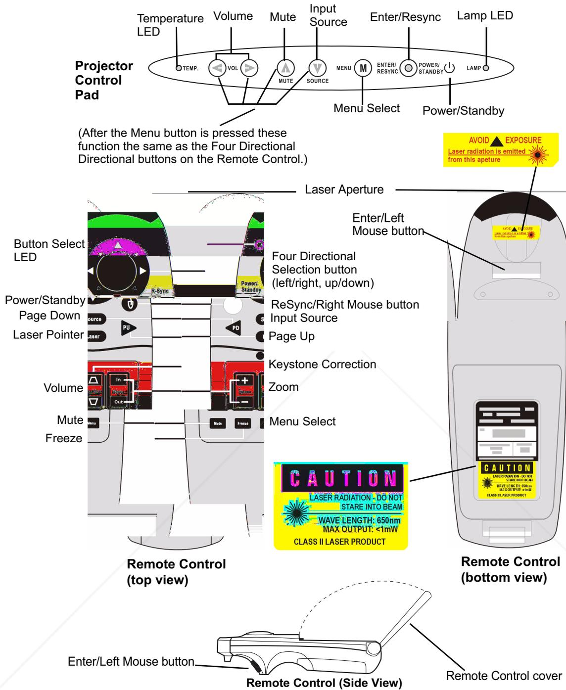
Figure 5: Projector Control Pad and Remote Control
