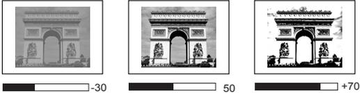
2. **Brightness:** Adjusts the brightness of the image. The higher the value, the brighter the image. And lower the value, the darker the image. Adjust this control so the black areas of the image appear as black and that detail in the dark areas is visible.
