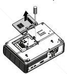
Loosen the two captive screws that secure the lamp.
