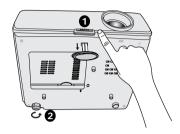
If the projector is not placed on a flat surface or the screen and the projector are not perpendicular to each other, the projected image becomes trapezoidal. To correct this situation, see "Correcting keystone" on page 31 for details.
