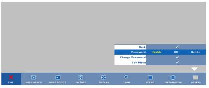
**b** Enabling the Password function will pop up a character screen, key in a 4-digit number from the screen and press on the control panel or press Enter button on the remote control.
