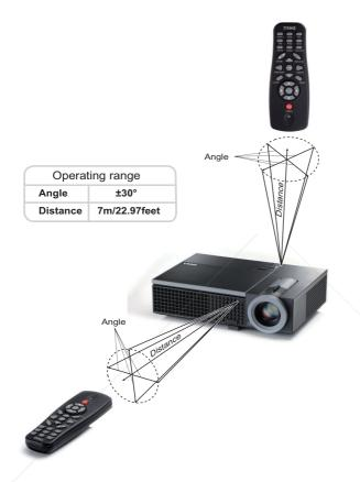
NOTE: Actual operating range may slightly differ from the diagram. Weak batteries will also prevent the remote control from properly operating the projector. The TRUSTED SOURCE FOR PROJECTOR LAMPS AND ACCESSORIES
