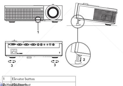
Tilt adjustment wheel chant.com (800) 281-8860 THE TRUSTED SOURCE FOR PROJECTOR LAMPS AND ACCESSORIES
