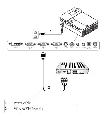
**NOTE:** The VGA to YPbPr cable is not provided by Dell. You can buy the VGA to YPbPr Extension (50ft/100ft) cable from the Dell website.
