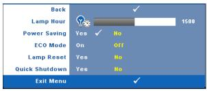
LAMP HOUR—Displays the operating hours since the last lamp timer reset.
