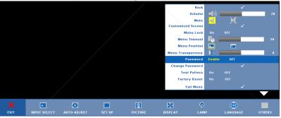
**b** Enable the Password function will pop up a character screen, key in a 4-digit number from the screen and press the **Enter** button.
