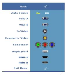
**AUTO SOURCE—**Select On (the default option) to autodetect the available input signals. If you press the Source button when the projector is on, it automatically finds the next available input signal. Select Off to lock the current input signal. If you press the Source button when the Auto Source mode is set to Off, you can manually select the input signal.
