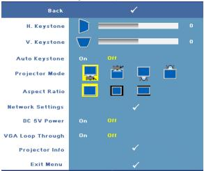
**H. KEYSTONE**—Adjusts the image distortion caused by horizontal shifting of the projector orientation.
