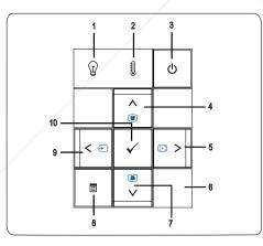
FixYourDLP.comP warning light Discount-Merchain If the LAMP light is solid amber, replace the lamp. If the LAMP light is blinking amber, the lamp driver or color wheel have failed and the projector automatically shuts down IF the ORIES problem persists, contact Dell<sup>™</sup>.
