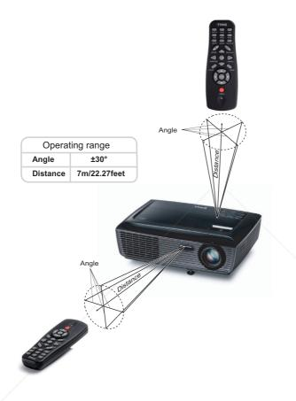
**NOTE:** Actual operating range may slightly differ from the diagram. Weak batteries will also prevent the remote control from properly operating the
