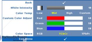
WHITE INTENSITY—Use  $\triangleleft$  and  $\geqslant$  to adjust the display white intensity. 281-8860
