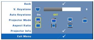
**V. KEYSTONE**—Adjusts the image distortion caused by tilting the projector.
