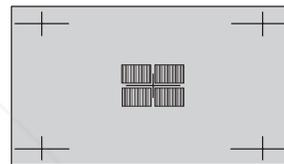
2. Press **ENTER** to display test pattern 2 and adjust the focus with the **Focus ring** again.
