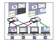
If you press the [MULTI-LIVE SELECT] button once or twice when index windows are displayed on the projection screen, the screen will switch over to a full screen display.
