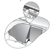
Do not insert your hand into the projector when the lamp is removed. If you touch the optical components inside, it could cause blurred images.
