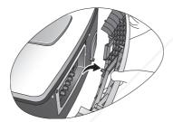
Manage all the connected cables within the indentation of the cable connector-panel cover and attach it to the projector securely.
