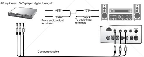
The RCA type component video sockets are provided for connection to video output devices. If you have a BNC type component video cable, you can alternatively connect through the BNC component video sockets.
