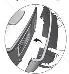
Turn the projector over again. Tighten the screws 6. to hold the cable connector-panel cover and the projector on both sides.
