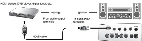
You should also connect the separate audio cable to a suitable audio amplifier.
