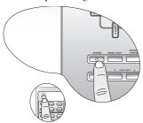
Remove the filter cover by gently lifting the loosened cover vertically upwards and then away from the projector body.
