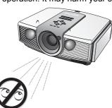
10. Do not operate the projector lamp beyond the rated lamp life. Excessive operation of lamps beyond the rated life could cause a lamp to break on rare occasions.
