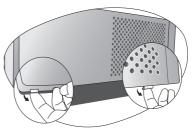
Remove the dust filter grill by pulling the tab outwards and away from the projector.
