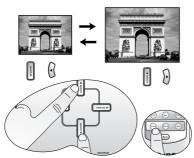
1. Adjust the projected image to the size that you need 2. Then sharpen the image by using the focus buttons. When the **FOCUS** button is pressed, an adjustment bar Focus displays on the screen. To further adjust the image clarity, press the ◀ or ▶ button on the projector or remote control.
