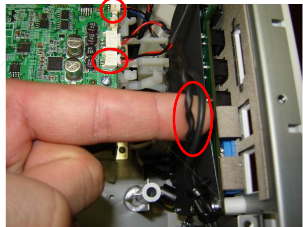
Arrange the wires as picture when you assemble it.
