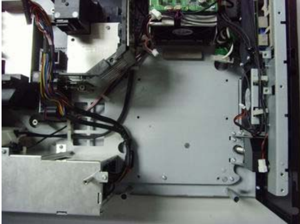
The Lens Shift / motor module off.
