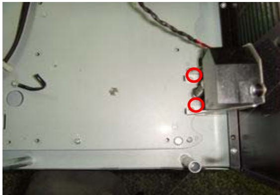
Remove the two screws and take away the L speaker.
