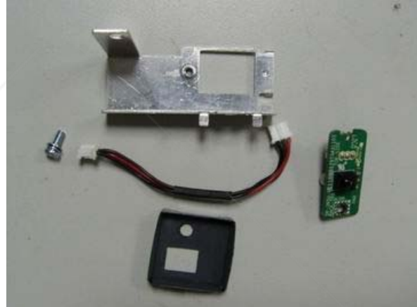
Disassemble the back IR assy.
