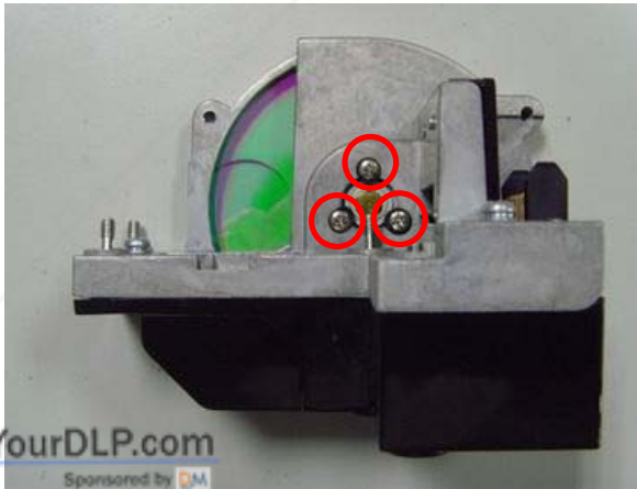
Remove the three screws and take this case away.
