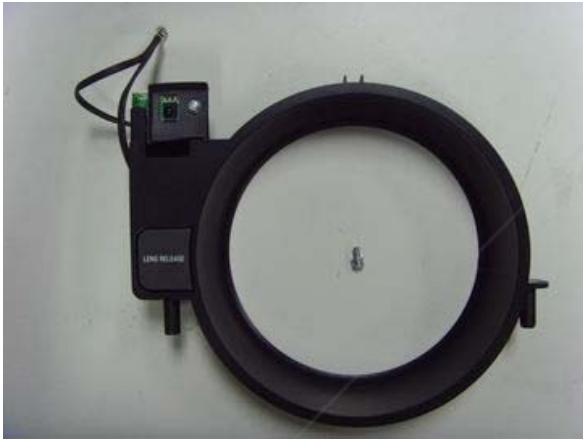
Disassemble the Lens cap & IR Assy.
