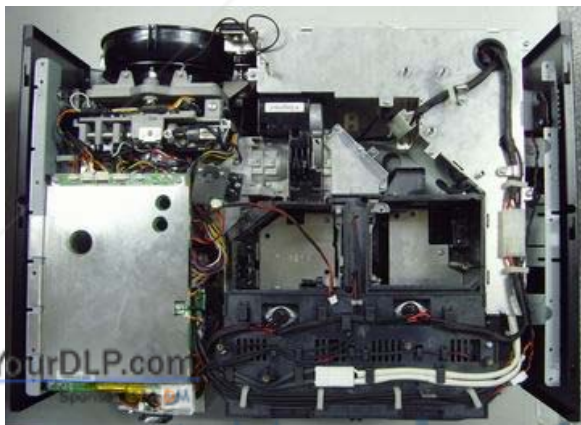
Then remove the top cover shield.
