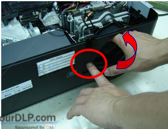
Push the Lens release button, Turn anti-Clockwise and pulled the lens away.
