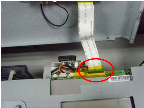
Remove the FCC Cable from the keypad side.
