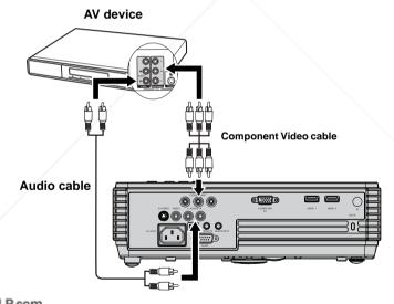
if the selected video image is not displayed after the projector is turned on and the correct video source has been selected, check that the Video source device is turned on and operating correctly. Also check that the signal cables have been connected correctly.
