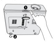
If the projector is not placed on a flat surface or the screen and the projector are not perpendicular to each other, the projected image becomes trapezoidal. To correct this situation, see "Correcting keystone" on page 31 for details.
