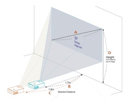
The table below shows how to achieve a desired image size by adjusting either the position or the zoom ring. For example: to obtain an image size of 50" set the projector at a distance 1.7 m and 1.8 m from the screen and adjust the zoom level accordingly.
