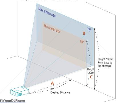
S (Figure: Fixed distance with different zoom and screen size. 300) 281-8860
