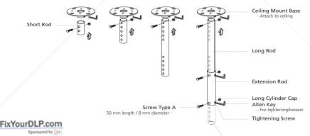
3 Use the appropriate number of screws for the projector size to attach the projector to the ceiling mount bracket.
