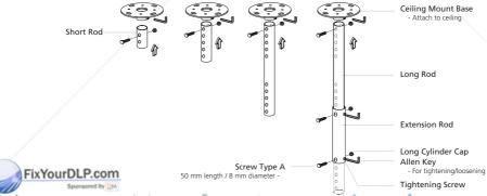
3 Use the appropriate number of screws for the projector size to attach the projector to the ceiling mount bracket.
