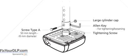
5 Adjust the angle and positioning as necessary.
