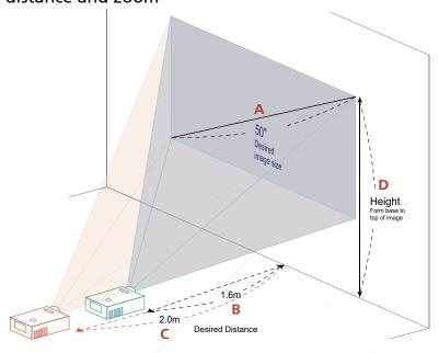
The table below shows how to achieve a desired image size by adjusting either the position or the zoom ring. For example: to obtain an image size of 50" set the projector at a distance 1.6 m and 2.0 m from the screen and adjust the zoom level accordingly.
