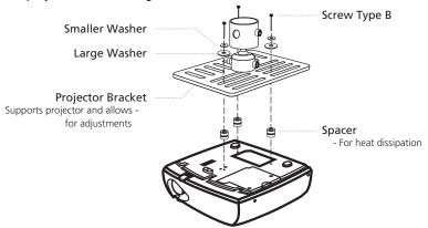
**Note:** It is recommended that you keep a reasonable space between the bracket and the projector to allow for proper heat distribution. Use two washers for extra support, if deemed necessary.
