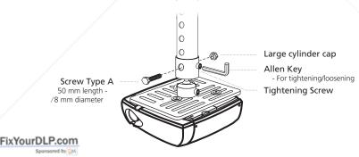
5 Adjust the angle and positioning as necessary.
