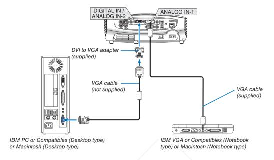
NOTE: When the DVI to VGA adapter is not to be used for an extended period of time, remove it from the projector. Failure to do so may cause damage to the connector of the projector.
