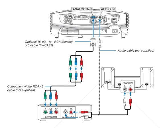
A component signal will be automatically displayed. If not, from the menu, select [Setup]  $\rightarrow$  [Options(1)]  $\rightarrow$  [Input signal select] or [Computer 2 (Analog)]  $\rightarrow$  [Computer 1], and then select [COMPONENT].
