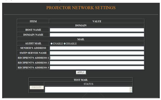
This option notifies your computer of an error message via e-mail when using wired LAN. An error message notification will be sent when the projector lamp has reached the end of its usable life or an error occurs in the projector.
