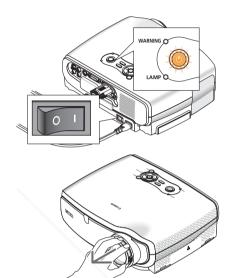
3. Press the POWER button on the projector cabinet or the POWER button on the remote control for about 1 second.
