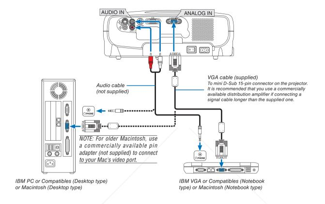
NOTE: Use an audio cable without a built-in resistor. Using an audio cable with a built-in resistor turns down the sound.
