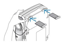
NOTE: Do not wash the filter with soap and water. Soap and water will damage the filter membrane. Before replacing the filter, remove dust and dirt from the projector cabinet. Keep out dust and dirt during filter replacement.
