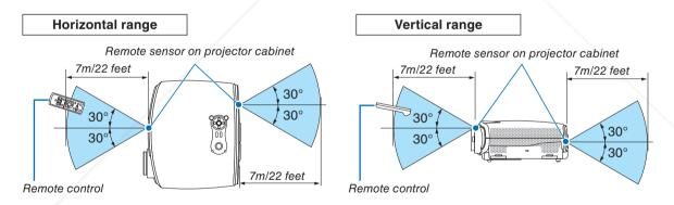
NOTE: The LV-7260 and LV-X7 do not have the remote sensor on the rear panel.
