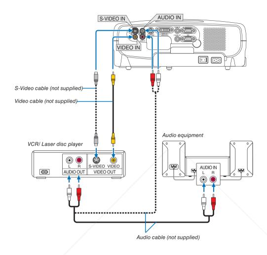
NOTE: The AUDIO IN L/MONO and R jacks (RCA) are shared between the Video and S-Video inputs.
