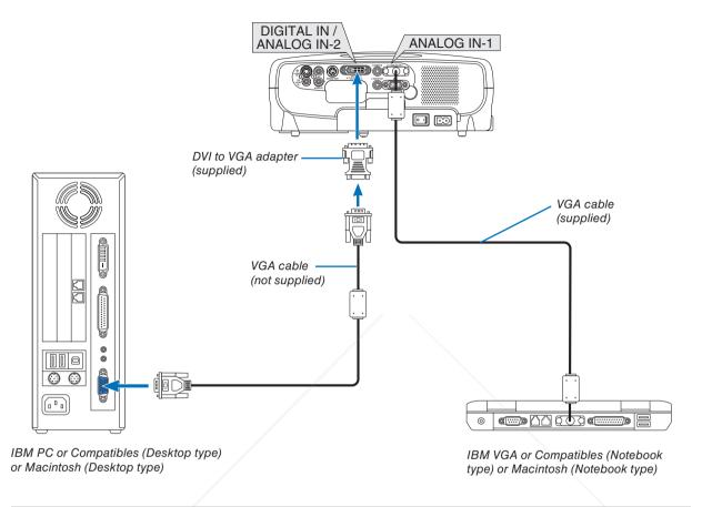
NOTE: When the DVI to VGA adapter is not to be used for an extended period of time, remove it from the projector. Failure to do so may cause damage to the connector of the projector.
