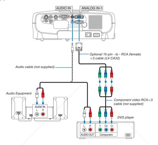
A component signal will be automatically displayed. If not, from the menu, select [Setup]  $\rightarrow$  [Input signal select]  $\rightarrow$  [Computer 1] or [Computer 2 (Analog)] ([Computer] on LV-7260/LV-X7)  $\rightarrow$  [COMPONENT].
