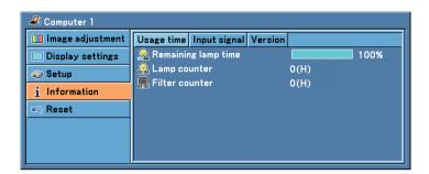
[Remaining lamp time] (%)\* [Filter counter] (H) [Lamp counter] (H)
