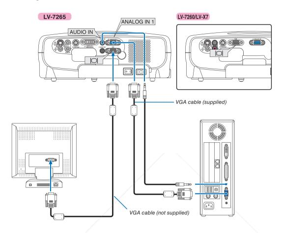
You can connect a separate, external monitor to your projector to simultaneously view on a monitor the RGB analog image you're projecting.
