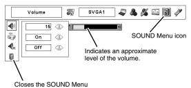
Built-in SP. 0 (800) 281-8860 Press the POINT LEFT/RIGHT buttons to switch the built-in speaker On or Off. AMPS AND ACCESSORIES  $(\mathbf{x}_{0})$ Mute
