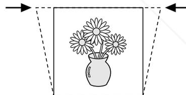
When ▼ is pressed, the lower part of the image is corrected.
