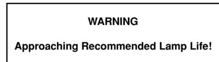
The lamp will fail to light and the POWER-ON, TEMP and LAMP monitors will flash about 100 hours after this message is displayed.
