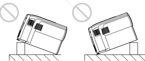
Do not install the unit other than on the floor. Do not adjust the height of the projector except the use of the adjuster.
