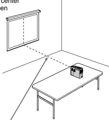
The distance between the lens and the screen varies depending on the size of the screen. Use the following table as a guide.
