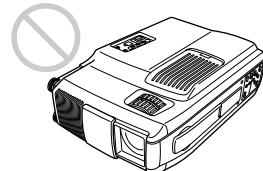
Avoid using as the unit topples over on its side. It may cause malfunction.
