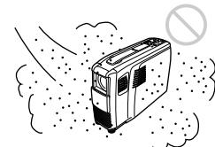
Avoid installing the unit in a location where there is a lot of dust; otherwise, the air filter will be obstructed. The dust blocking the air through the filter may cause raising the internal heat of the projector. Clean it up periodically.
