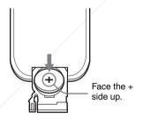
**3** Put the lithium battery holder back into the Remote Commander. FixYourDLP.com
