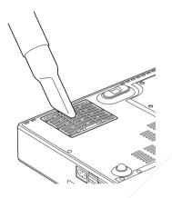
When it becomes difficult to remove the dust from the filter with a vacuum cleaner, remove the air filter and wash it.
